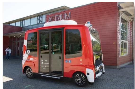
Figure 67 - Electric bi-directional driverless vehicle used for shuttle services
